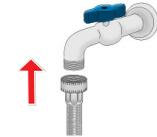
17) Hand tighten couplings, then use pliers to make an additional 1/4" turn clockwise. **Do not over-tighten couplings, as damage can result.**
